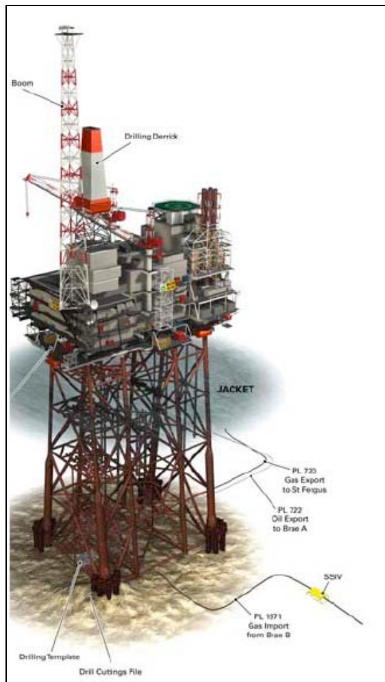
Figure 3.4. Example of a steel jacket: the four-legged tubular steel Miller platform (BP, 2008).
