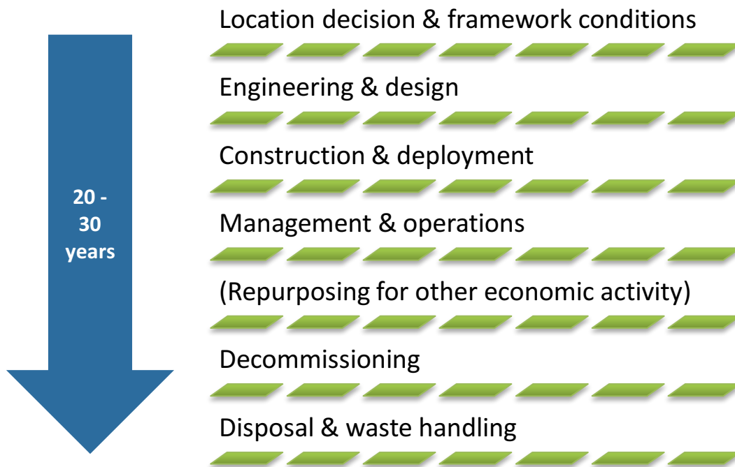
Figure 3.1. Illustration of a typical offshore installation life cycle.
